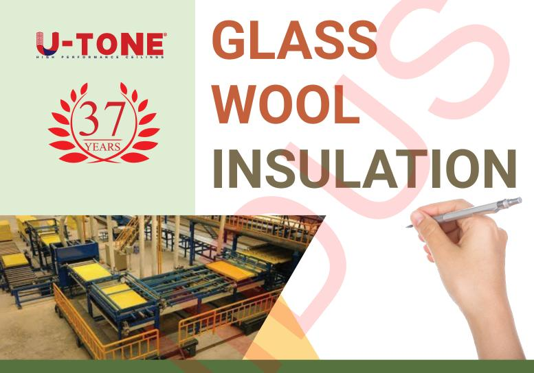
U-tone Glasswool is a soft, lightweight, gold in color compressible insulation material consisting of fine, long, inorganic glass fibers bonded together by a high-temperature binder. U-Tone Glasswool is available in rolls, slabs, and blankets and with a wide range of factory-applied facings which include reinforced aluminum foil, fiberglass tissue, etc.
